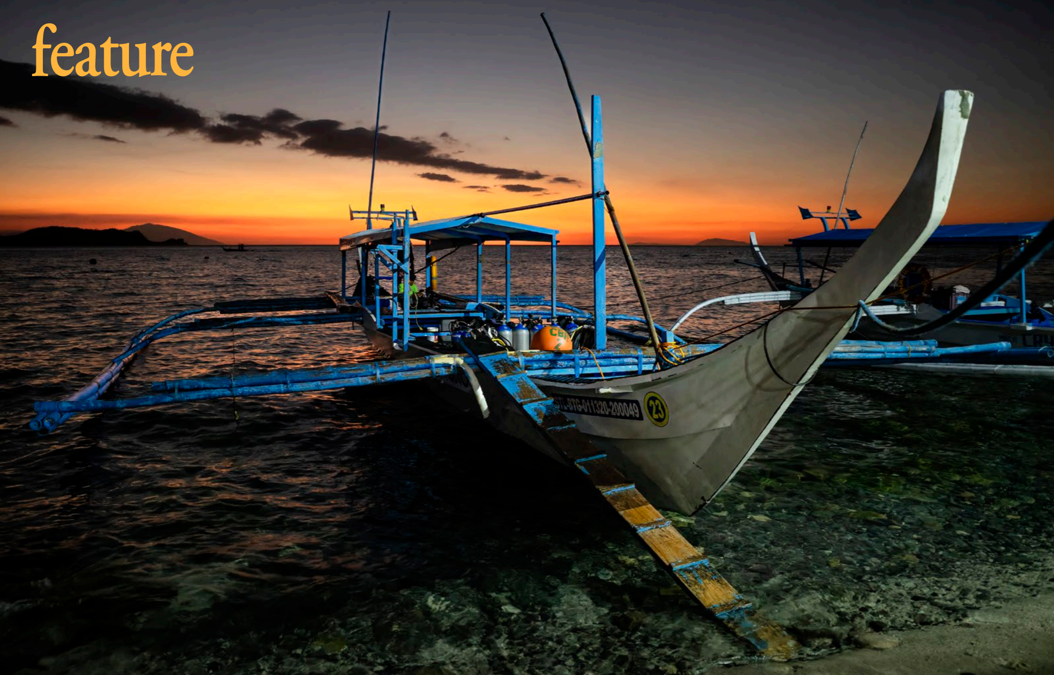
Traditional bangka boat adapted for diving, at the start of the “night shift” (above). Getting the “pumpkin” ready (right). This plastic orange buoy with its own video light supports the 25m-long, weighted downline, drifts with the current, and is easily followed by the divers.
