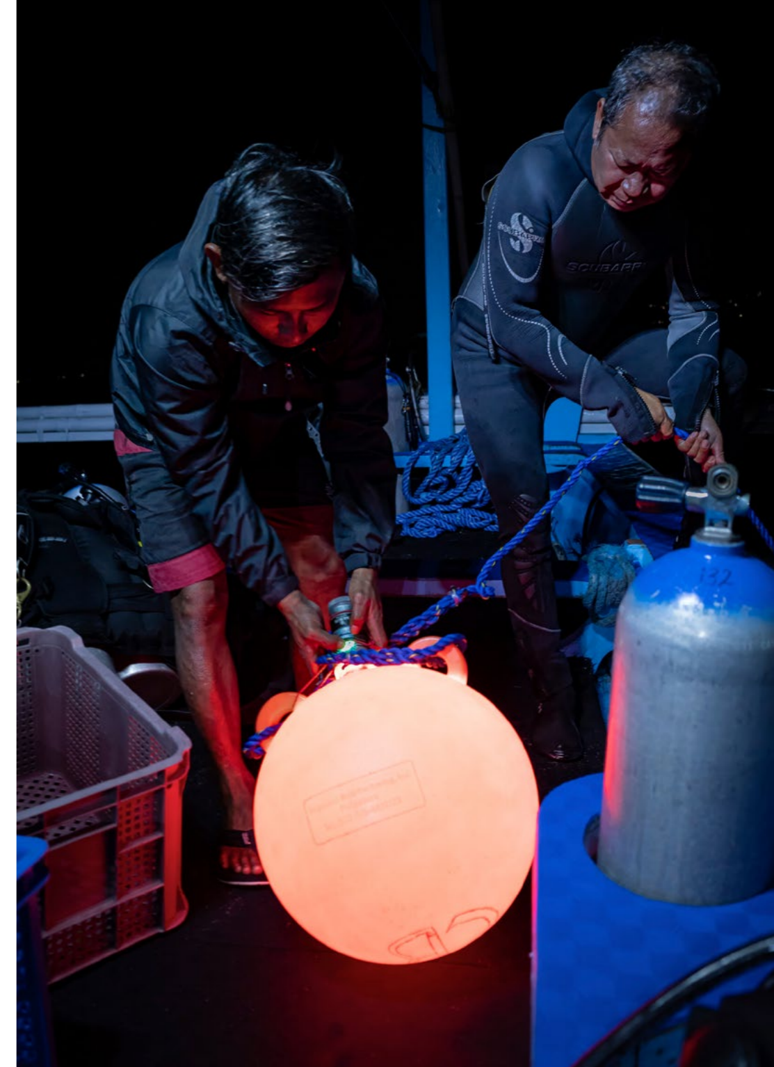
Traditional bangka boat adapted for diving, at the start of the “night shift” (above). Getting the “pumpkin” ready (right). This plastic orange buoy with its own video light supports the 25m-long, weighted downline, drifts with the current, and is easily followed by the divers.
