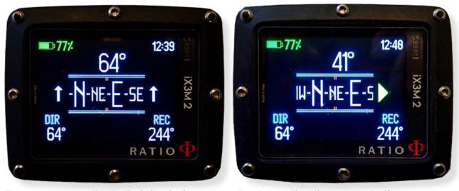
The compass on the Ratio iX3M 2 dive computer shows direction on and off course.
