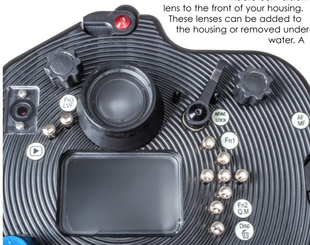
A housing should allow access to all important camera controls.
