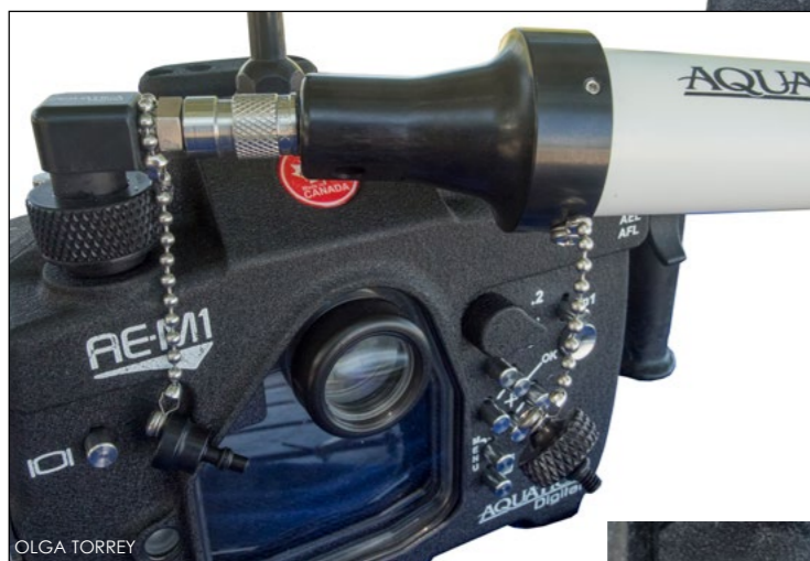
Vacuum valve on housing (above); Creating a vacuum to check for leaks (left)
