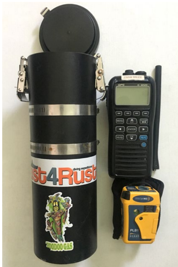
Housing with 6-watt VHF radio (with DSC function and GPS data) and PLB
