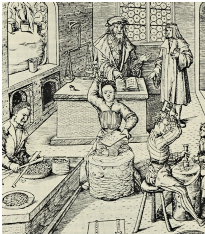
A 16th century woodcut provides a glimpse into the workings of a mint; blanks being cut from sheets of silver, struck into coins, weighed and documented
