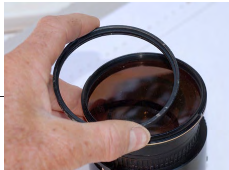
Depending on your subject, you either attach the filter in front of the lens (right), or you trim it to fit to slide in behind the lens (top)
