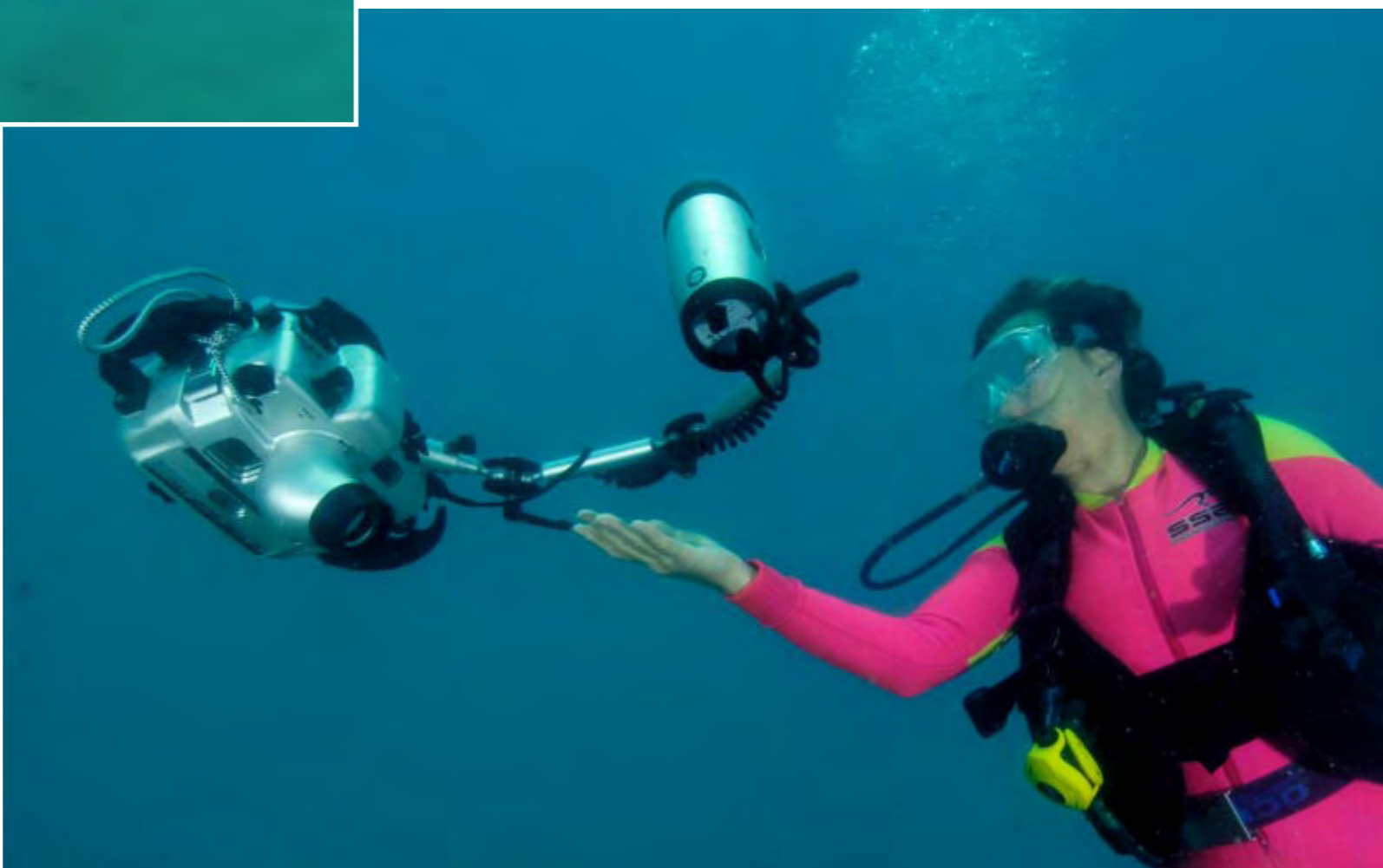
The complete rig should have less than 250 grams of negative or positive buoyancy
