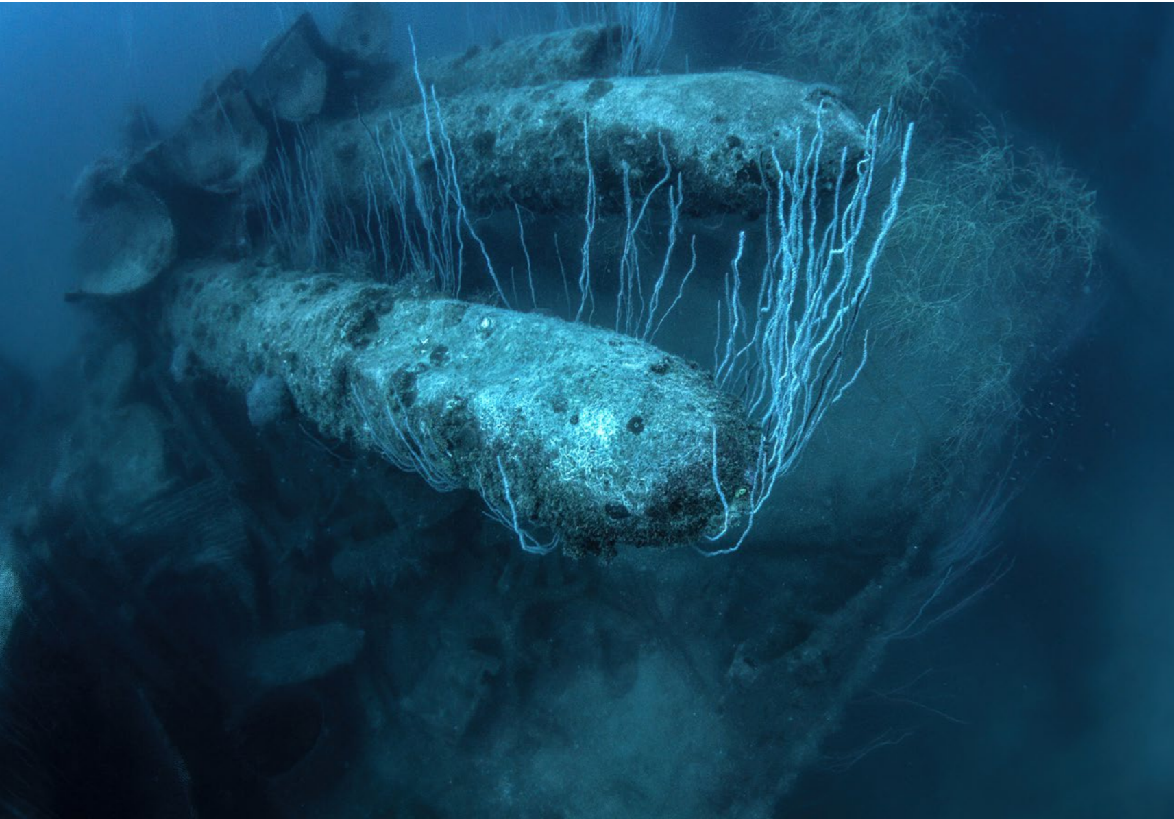
Torpedo launcher with torpedoes (above) and gun (right and top right) on USS Lamson
