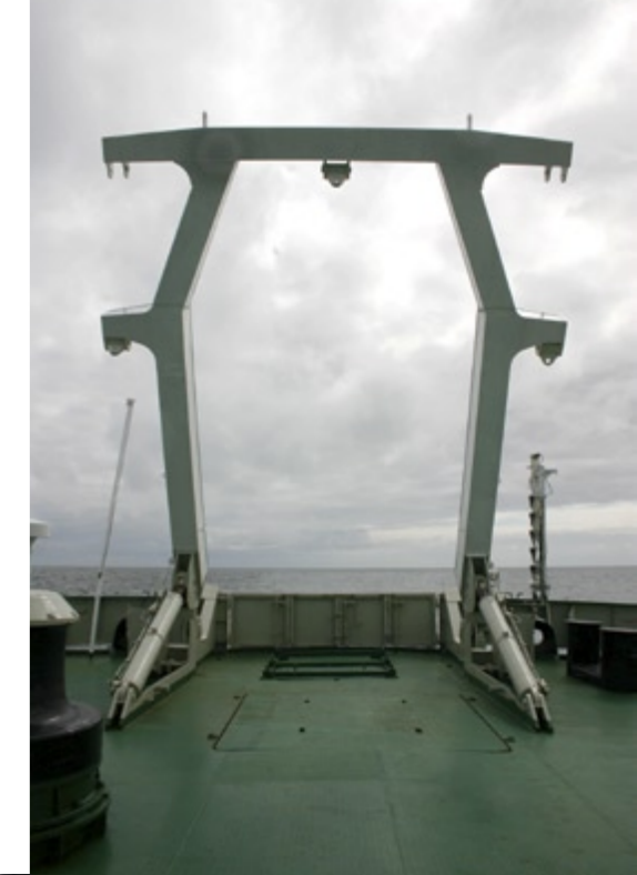
The P-Frame, a lifting device on the stern
