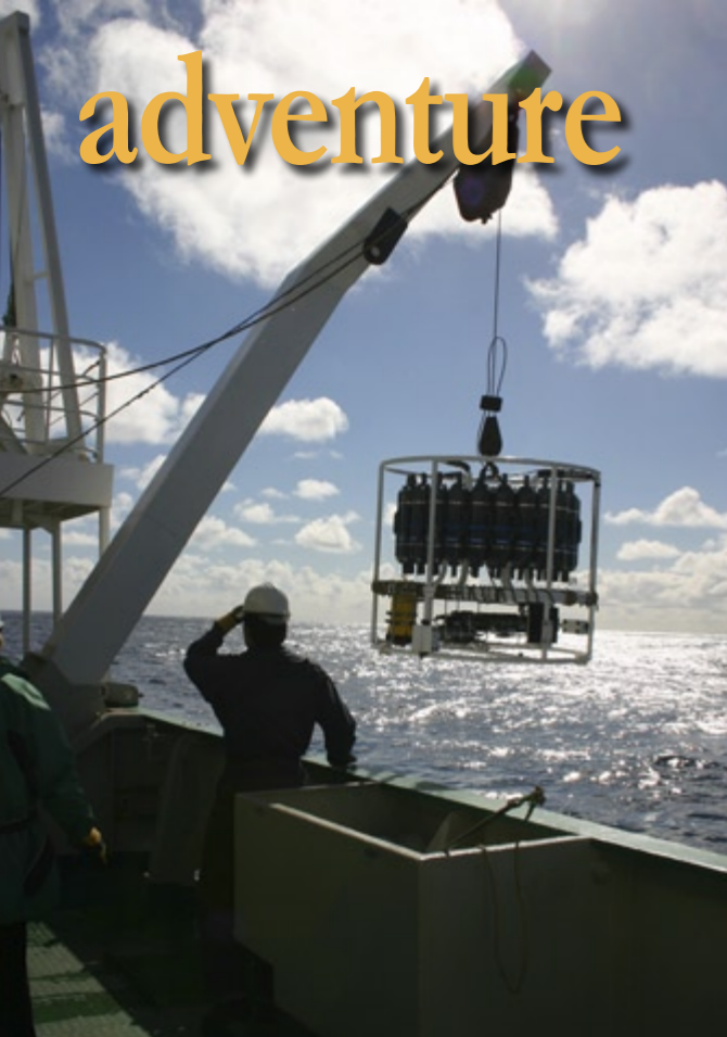
LEFT: Carousel deployment BELOW: Water sampling
