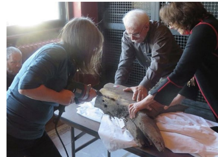
Sampling a crutch timber from the Sparrow-Hawk for tree-ring analysis
