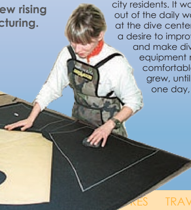
Dive System worker cuts out pattern pieces for the semi-drysuit
