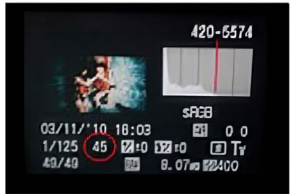
Figure 10. When bracketing exposures, check the histogram and “expose to the right,” as shown.
