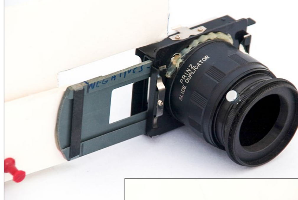
Figure 11. Insert the negative carrier fully into the copier (above) and insert negatives, emulsion side away, pinching the film slightly (right).
