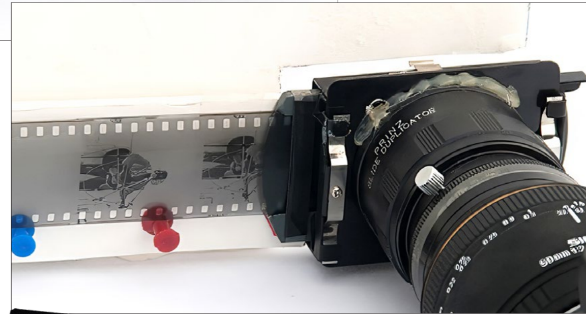
Figure 11. Insert the negative carrier fully into the copier (above) and insert negatives, emulsion side away, pinching the film slightly (right).
